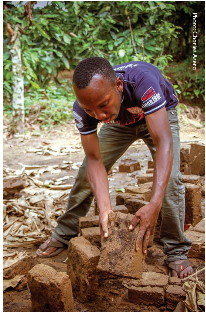
A young man in Uganda works on his masonry business, molding and baking bricks to build houses and retaining walls.
